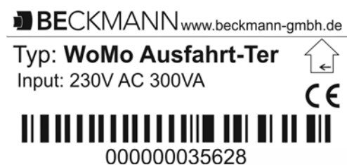
Fig. 1-4 Name plate of RV exit terminal with ticket reader
