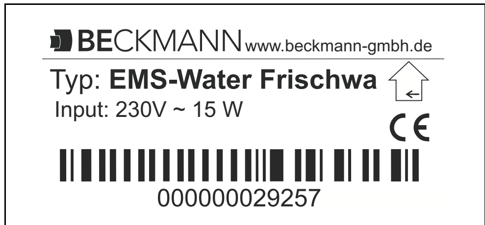
Fig. 1-1 Name plate of fresh water tower without trace heating
