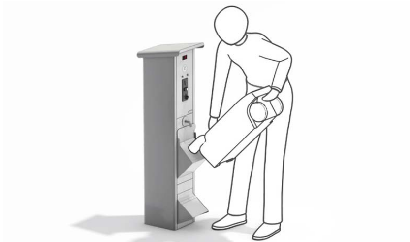
Fig. 6-16 Draining the waste water tank
