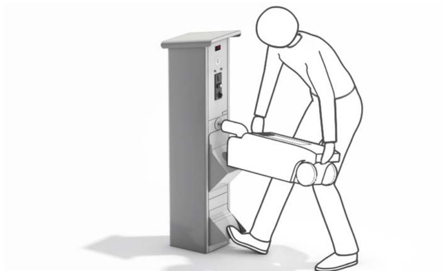
Fig. 6-17 Flushing the waste water tank
